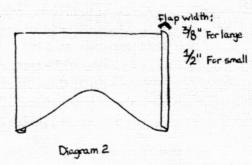
The next step is to use a convenient metal tube (an old water pipe works well) for forming the tin pieces into pipe shapes. Place the metal tube close to and parallel with one of the flapped sides of the tin. Then bend the tin over the tube slightly. Then move the tube away from the flap a little and again bend the tin over slightly. Continue this bending process across the 24 in. length of the tin (at the midpoint the tin can be turned over and
