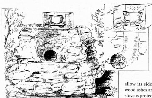
Now take the curved piece that was cut out of the 18 x 24 in. sheet of tin and make two cuts in it so it will slide into the horizontal tube about a third up from the bottom; the width of this piece will be fewer than 7 in. This makes a shelf for the firewood, which is placed on top. Finally, make a tin shield at least on three sides (the same height as the cooking pot) that will surround the cooking pot and
