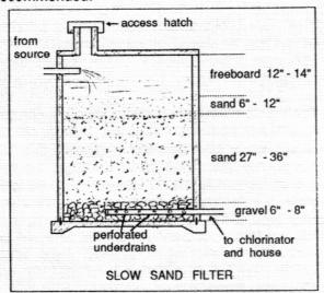
Sand filters eventually clog and require periodic maintenance. Rapid sand filters are cleaned by backwashing: pumping clean water back through the filter to wash out the fine particles. With a slow sand filter, the top half inch or so of sand is removed. This is generally roasted to remove contaminants and saved for later return. After six inches or so have been removed, clean sand should be added to the bottom of the filter by double digging.
