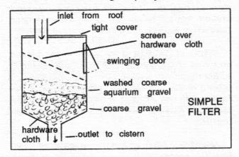
It is ideal for small water systems serving 25-3,000 people, but can be custom built from concrete materials to accommodate larger numbers. Size and cost depend upon water demand. Some method of disinfection after sand filtering is generally recommended.
